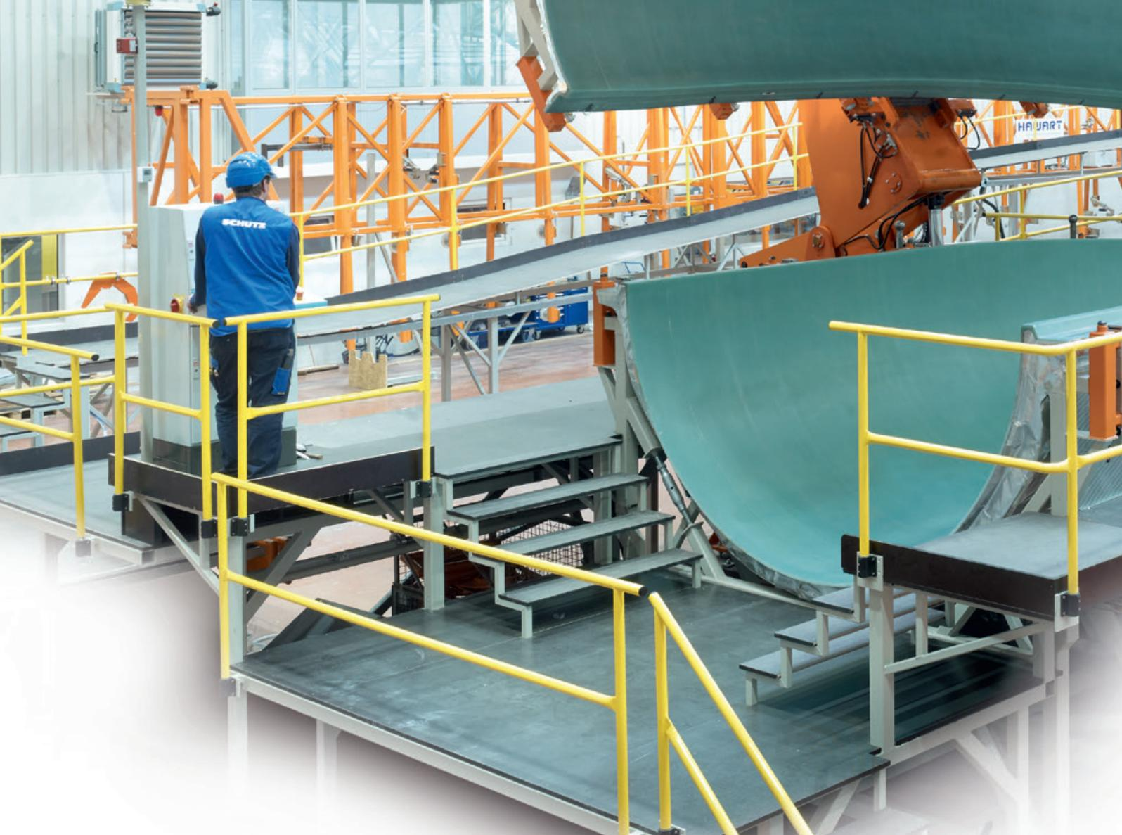
Impressive: the giant main mould with integrated electric heating for making millimetre-precise wind turbine blades.
